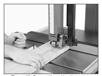
Figure 40. Crosscutting with miter gauge.
